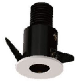
DM-01035F (High 50 mm) Trim Ø 35 mm Cut-out Ø 30 mm
