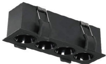
DF-08154F (High 56 mm) Trim 154*49 mm Cut-out 145*40 mm
