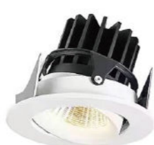
DE-01092C (High 70 mm) Trim Ø 92 mm Cut-out Ø 78 mm
