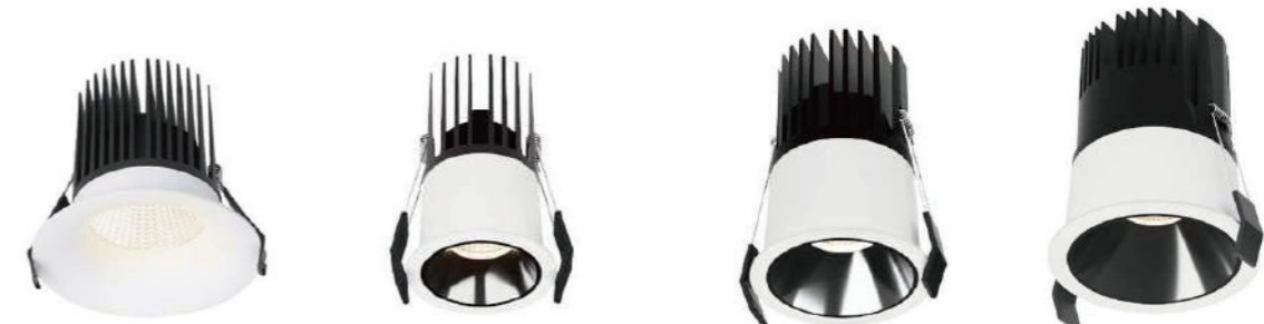
DR-15135A (High 119 mm) Trim Ø 135 mm Cut-out Ø 108 mm DR-03063F (High 95 mm) Trim Ø 63 mm Cut-out Ø 55 mm DR-03085F (High 120 mm) Trim Ø 85 mm Cut-out Ø 75 mm DR-03110F (High 138 mm) Trim Ø 110 mm Cut-out Ø 95 mm
