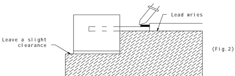
Regarding tinning the leads, compound made of tin ,copper and sliver is proposed with the temperature of 260°C. The proportion of the alloyed solution is 95.5% tin, 3.5 % copper, 0.5% silver. The time of tinning is 3 seconds.
