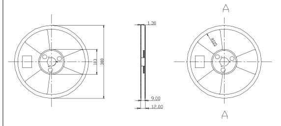
Carrier Tape Dimensions: Loaded Quantity 4000 pcs Per Reel.
