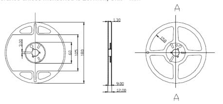
Note: Carrier Tape Dimensions: Loaded Quantity 4000 pcs Per Reel.
