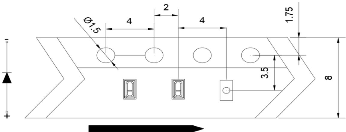
Note: Tolerance unless mentioned is  $\pm 0.1$ mm; Unit = mm
