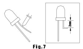
2) Forming lead should be carried our prior to soldering and never during or after soldering.
