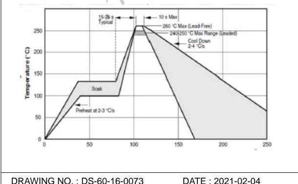
7) Recommended Wave Soldering Profile.
