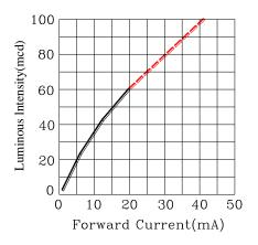
Fig.3 Luminous Intensity vs.Forward Current
