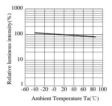
Fig.5 Luminous Intensity vs. Ambient Temperature
