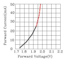
Fig.2 Forward Current vs.Forward Voltage
