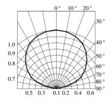
Fig.7 Relative Intensity vs. Angle
