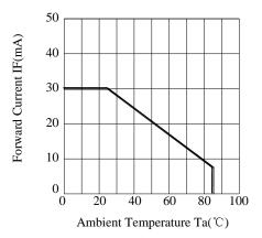
Fig.6 Forward Current Derating Curve
