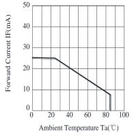
Fig.6 Forward Current Derating Curve
