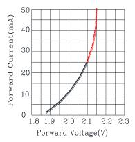
Fig.2 Forward Current vs.Forward Voltage
