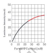
Fig.3 Luminous Intensity vs.Forward Current
