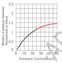
Fig.4 Relative Luminous Intensity vs.Forward Current
