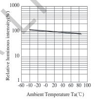
Fig.5 Luminous Intensity vs. Ambient Temperature
