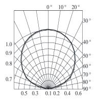
Fig.7 Relative Intensity vs.Angle
