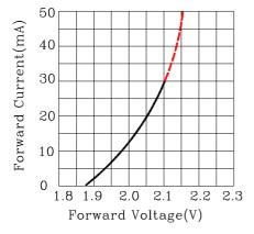
Fig.2 Forward Current vs.Forward Voltage
