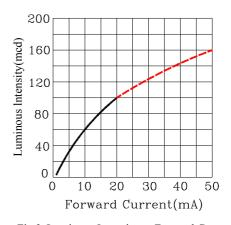
Fig.3 Luminous Intensity vs.Forward Current
