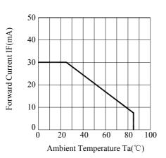
Fig.6 Forward Current Derating Curve
