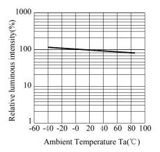
Fig.5 Luminous Intensity vs. Ambient Temperature
