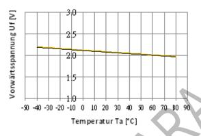
Fig3 Ambient Temperature vs.Forward Voltage
