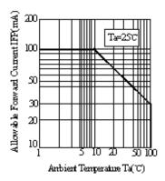
Fig6 Forward Current Derating Curve
