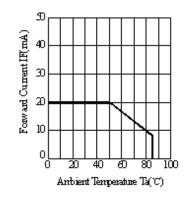
Fig 4 Forward Current Derating Curve
