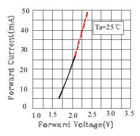
Fig. 1 Forward Current vs. Forward Voltage
