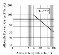
Fig.4 Forward Current Derating Curve
