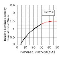
Fig.2 Relative Luminous Intensity vs.Forward Current
