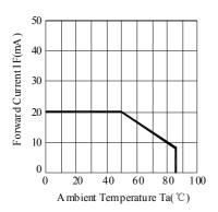
Fig.5 Forward Current Derating Curve
