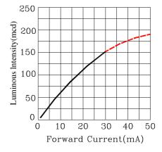
Fig.2 Luminous Intensity vs.Forward Current
