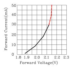
Fig.1 Forward Current vs.Forward Voltage
