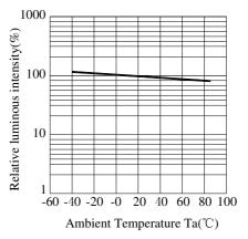
Fig.4 Luminous Intensity vs. Ambient Temperature
