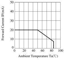
Fig.5 Forward Current Derating Curve
