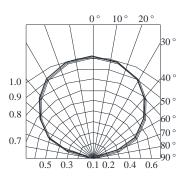
Fig.7 Relative Intensity vs.Angle
