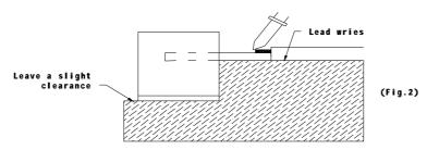
Regarding solution in the tinning oven for product-tinning, compound sub-solution made of tin & copper and sliver is proposed with the temperature of Celsius 260. The proportion of the alloyed solution is tin 95.5: copper 3.5: silver 0.5 by percentage. The time of tinning is constantly 3 seconds.
