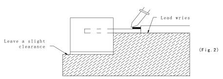
Regarding tinning the leads, compound made of tin ,copper and sliver is proposed with the temperature of  $260^{\circ}$ C. The proportion of the alloyed solution is 95.5% tin, 3.5 % copper, 0.5% silver. The time of tinning is 3 seconds.
