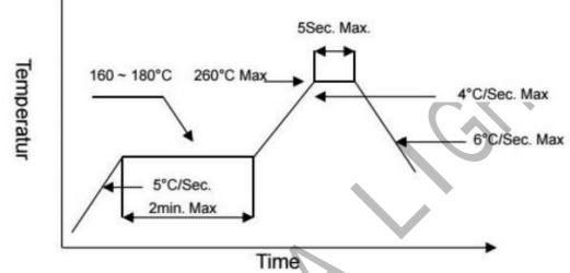
3. DIP soldering (Wave Soldering) :
